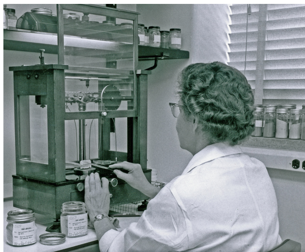
Figure 4.5: Elizabeth Linden using an analytical balance to prepare samples for analysis in the Analytical Laboratory. UA 16.18. Michigan State University Archives and Historical Collections, East Lansing, MI.
