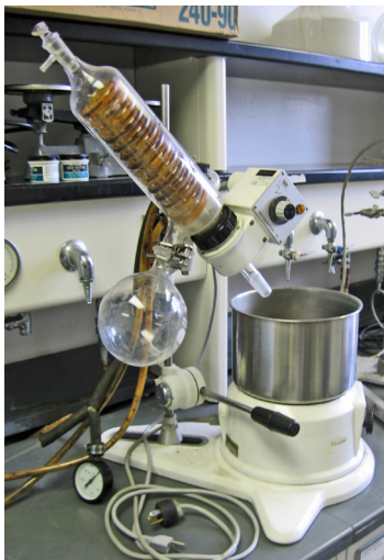
Buchi Rotary Evaporator, YC 1158, was purchased by the Plant Research Laboratory in June 1969 for $594. Courtesy of Robert Keck, MSU Service. Courtesy of Suzanne Hoffman-Benning.
