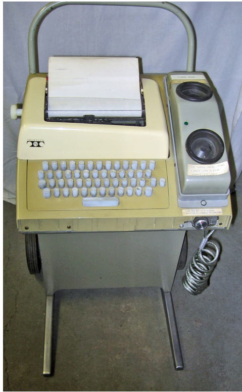
Figure 4.22: Teletype with acoustical coupler used to transmit data to the CDC 3600 Computer via the telephone. Photograph courtesy of the Michigan State University Museum Historical Collections.
