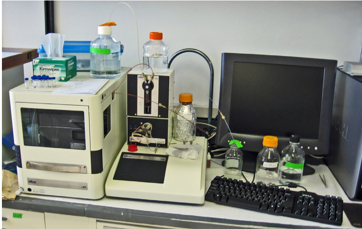
Reichert Surface Plasmon Resonance Spectrometer System, 100334, was purchased by the Department of Biochemistry and Molecular Biology in January 2010 for $70,000. Courtesy of Robert Keck, MSU Services. Photograph courtesy of Charles Hoogstraten.
