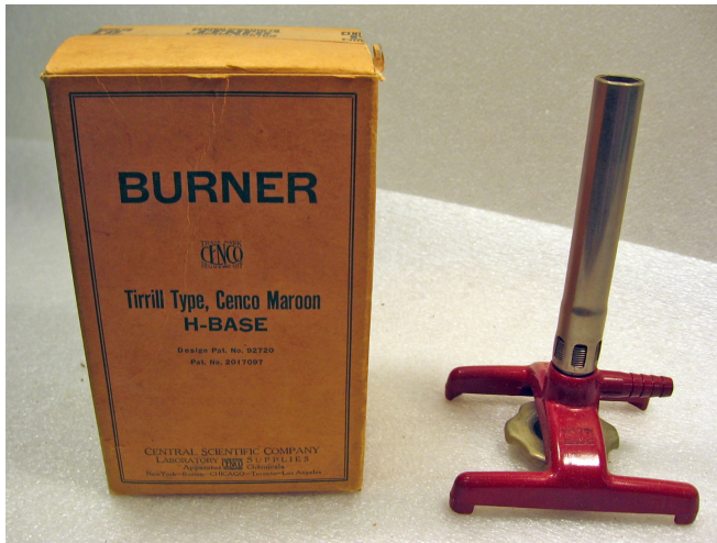
Bunsen Burner, Tirrel Type, H-Base, and its container. It was made by the Central Scientific Co. Courtesy of the Michigan State University Museum Historical Collections.
