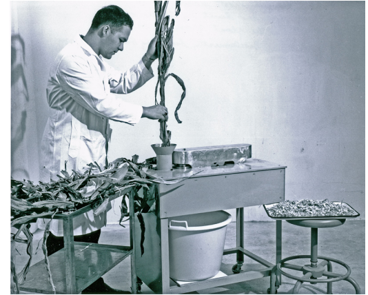
Figure 4.3: Vaughn Snook using a grinder built by Lester Hoag to grind corn stalk in the plant growth chambers in the basement of the Biochemistry Building in 1965. UA 16.18. Michigan State University Archives and Historical Collections, East Lansing, MI.
