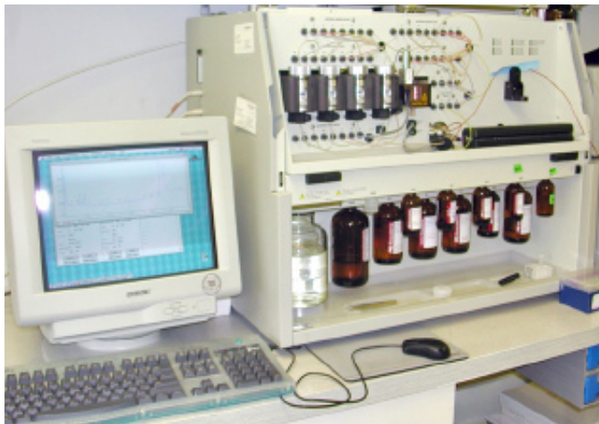
Figure 4.32: An Applied Biosystems Procise cLC494 Protein/Peptide Sequencer used by researchers in the Macromolecular Structure Core of the Research Technology Support Facility. Courtesy of Colleen Curry, Stacy Trzos and Joe Leykam, Research Technology Support Facility.
