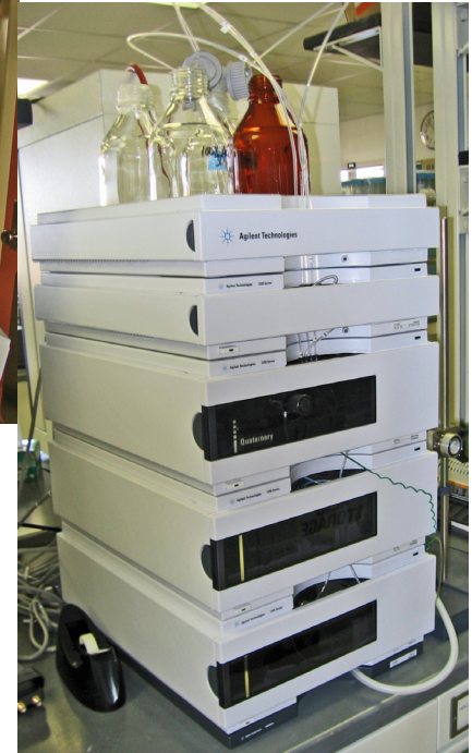
Agilent Technologies 1200 Series HPLC, 100067, was brought from Texas A & M University to the Department of Biochemistry and Molecular Biology in September 2009: value $11,538. Courtesy of Robert Keck, MSU Services. Photograph courtesy of Barbara Atshaves
