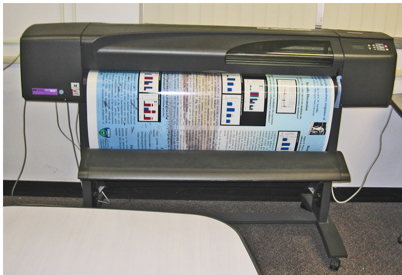
Figure 4.28: A view of the printer in the Macromolecular Computer Facility used to print 42 inch wide posters used for a variety of purposes, most importantly, posters used in scientific poster sessions. Courtesy of Kaillathe Padmanabhan.
