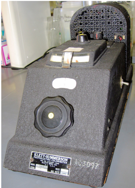
Klett Summerson Colorimeter, AC 3097, purchased by the Agricultural Chemistry Department in October 1956, for $227. Courtesy of Robert Keck, MSU Services.
