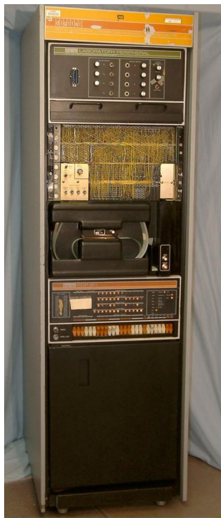
From top to bottom is the AX08 laboratory peripheral, DF32 disk drive, PC01 high speed paper tape, and the PDP-8/I computer.. http://www.pdp8.net/pdp8i/pics/8irack.shtml?med
