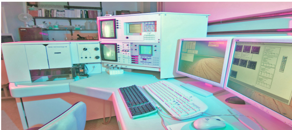
Figure 4.17: View of the Becton-Dickinson Vantage SE TurboSort flow cytometer currently in the Flow Cytometry Facility. The basic instrument was acquired in 1992 and upgraded to digital in 2002. Courtesy of Louis King,
